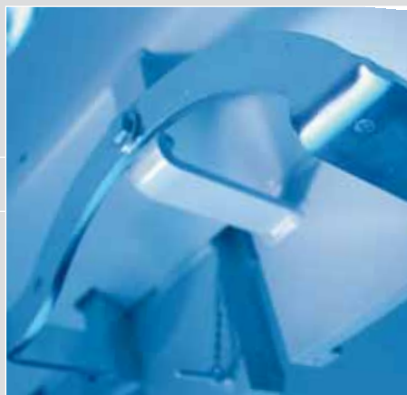
User friendly, easy-to-operate bracket used to activate the bale ejection device
